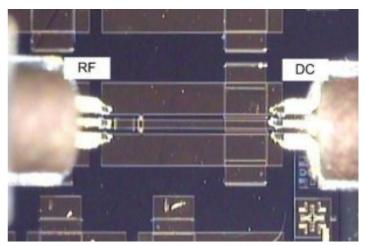
A microscope image of an RTD. [Image courtesy of University of Glasgow.]
