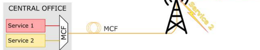
Fig. 4: Schematic showing backhaul and fronthaul signals carried over multicore fibre and based on TERAPOD UTC PDs from UCL.
